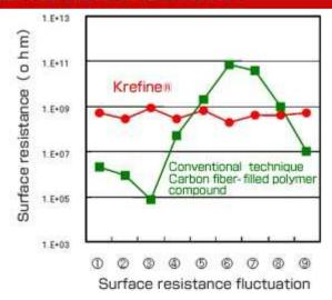
As illustrated in the graph above, Krefine's new technology results in consistent and controlled surface resistance for each point at specific levels within the range of 10<sup>6</sup> to 10<sup>11</sup> ohm on an injection molded specimen. The surface resistance of a carbon fiber reinforced compound however, is highly variable versus that of the Krefine molded part. This variability is due to uneven distribution of the carbon fiber at the parts
